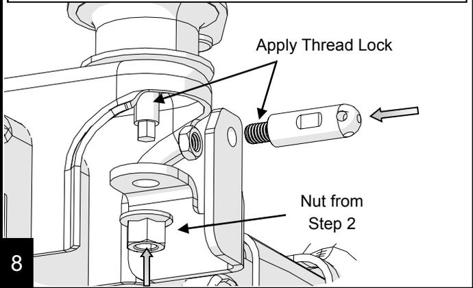
Torque the body mount to **80 ft-lb** and jam nut to **75 ft-lb**.
