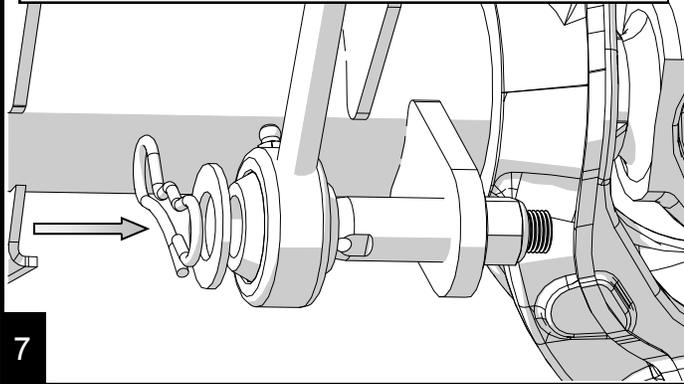
Remove the front body mount nut from the stud and slide on retaining bracket 600277. Then using the nut saved from Step 2 secure the bracket. Next insert stud 600503 into retaining bracket and install jam nut 73.
